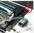
5. Install the bottom strip back and fix the two screws in the left side.
